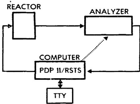
Fig. 1. Closed-loop system for automated chemical synthesis.
